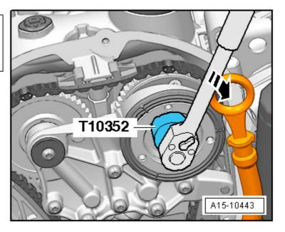
Remove bolts -arrows- and detach bearing saddle.
