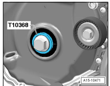
Use thrust piece -T10354- and bolt for vibration damper to pull in oil seal -arrow- onto stop.
