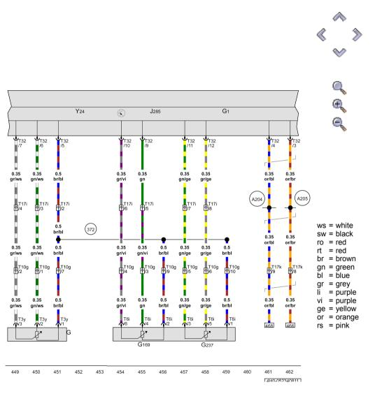
Fuel gauge, Fuel gauge sender 2, Fuel gauge sender 3, Control unit in dash panel insert
