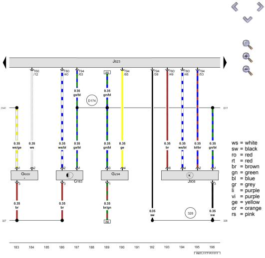
Hall sender 2, Brake servo pressure sensor, Regulating flap
