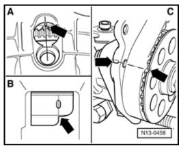
Insert counter-hold T10025 and loosen vibration damper and toothed belt pulley by loosening center bolt.
