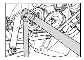
Insert counter-hold T10025 and tighten crankshaft vibration damper and toothed belt pulley center bolt to 460 Nm.
