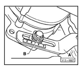
Tension V-belt by turning the tensioning nut -Bwith torque wrench Specification:
