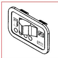
**A) PETROL-GAS AUTOMATIC CHANGEOVER MODE:** With changeover switch in its central position, vehicle starts up in petrol mode, then automatically changes over to gas. Changeover happens during deceleration or acceleration (according to the installer's set up), after exceeding a programmed rpm threshold and after a programmed rpm decrease, or after a deceleration.
