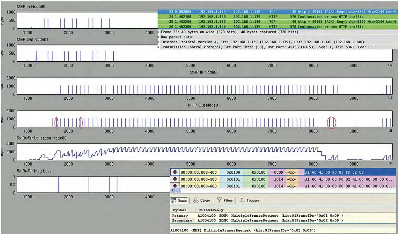
Figure 3. Evaluation of a TCP/IP and MHP data connection with different tools.
