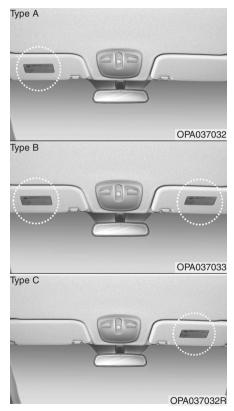
Air bag warning labels are attached to alert the driver and passengers of potential risk of air bag system.
