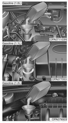
If it is near or at L, add enough oil to bring the level to F. Do not overfill.
