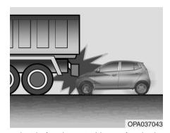
Just before impact, drivers often brake heavily. Such heavy braking lowers the front portion of the vehicle causing it to "ride" under a vehicle with a higher ground clearance. Air bags may not inflate in this "under-ride" situation because deceleration forces that are detected by sensors may be significantly reduced by such "under-ride" collisions.
