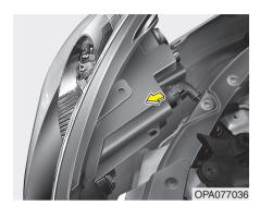
5. Disconnect the power connector from the back of the headlight assembly.
