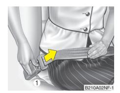
To release the seat belt: When you want to release the seat belt, press the button (1) in the locking buckle.
