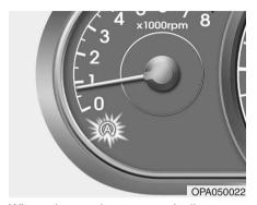
When the engine automatically stops, the "AUTO STOP" indicator on the cluster panel will illuminate.
