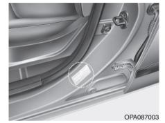
All specifications (sizes and pressures) can be found on a label attached to the vehicle.
