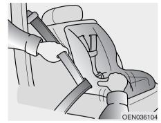
Buckle the seat belt and allow the seat belt to take up any slack. After installation of the child restraint system, try to move it in all directions to be sure the child restraint system is securely installed. If you need to tighten the belt, pull more webbing toward the retractor. When you unbuckle the seat belt and allow it to retract, the retractor will automatically revert back to its normal seated passenger emergency locking usage condition.
