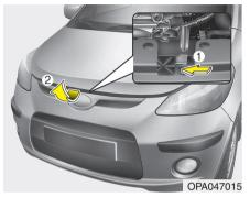
Go to the front of the vehicle, raise the hood slightly, pull the secondary latch (1) inside of the hood center and lift the hood (2).
