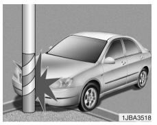
Air bags may not inflate if the vehicle collides with objects such as utility poles or trees, where the point of impact is concentrated to one area and the full force of the impact is not delivered to the sensors. C041100APA
