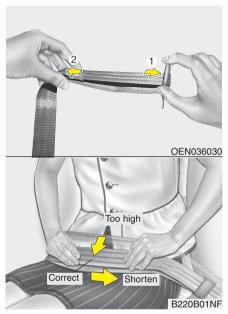
With a 2-point static type seat belt, the length must be adjusted manually so it fits snugly around your body. Fasten the belt and pull on the loose end to tighten. The belt should be placed as low as possible on your hips, not on your waist. If the belt is too high, it could increase the possibility of your being injured in an accident.
