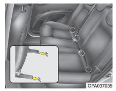
On each side of the rear seat, between the cushion and backrest, are located a pair of ISOFIX anchorage points together with a top tether mounting on the floor behind the rear seats. During the installation, the seat has to be engaged at the anchorage-points in a way you can hear it clicking (check by pulling!) and has to be fixed with the Top Tether-belt on the belonging point on the floor behind the rear seats.
