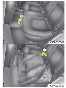
Lift the front portion of the seat cushion. Lift the rear portion of the seat cushion and stand the rear seat cushion vertically.
