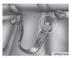
When using the rear center seat belt, the buckle with the "CENTER" mark must be used. (if equipped)
