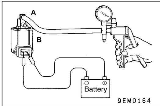
**PURGE CONTROL SOLENOID VALVE CHECK**
