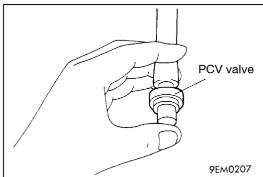
5. Place a finger at the opening of the PCV valve and check that vacuum of the intake manifold is felt.
