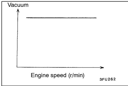
2. Start the engine and check that the vacuum remains fairly constant after racing the engine.
