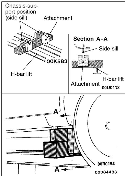
1. Place the vehicle on the H-bar lift (same direction).
