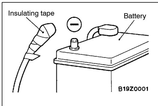
4. After disconnecting the battery cable, wait 60 seconds or more before proceeding with the following work. The SRS system is designed to retain enough voltage to deploy the air bag for a short time even after the battery has been disconnected, so serious injury may result from unintended air bag deployment if work is done on the SRS system immediately after the battery cables are disconnected.
