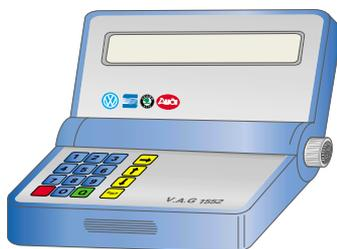
The fault reader V.A.G 1552 is as a compact second unit. Operation and function are identical to fault reader V.A.G 1551. Only the Print function has been dispensed with in order to achieve a compact unit.
