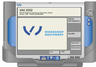
The market launch of the Vehicle Diagnostic and Service Information System VAS 5052 introduces a successor tester for the fault readers V.A.G 1551/1552.
