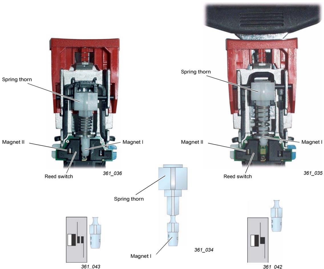
Two resistors are integrated in the circuit. Depending on the position of the reed switch, measurement takes place via one or both resistors. Based on the measured resistance value, the airbag control unit recognises whether the seat belt is fastened or not.
