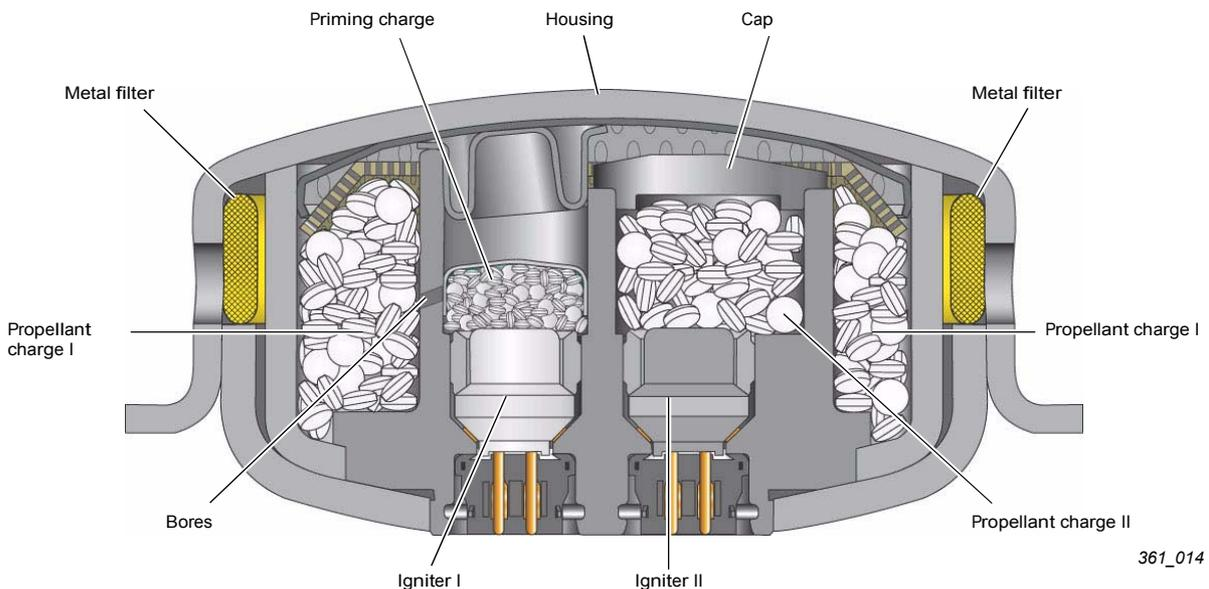
The driver's airbag gas generator is flexibly mounted in a rubber ring. This minimises any vibration at the steering wheel. The gas generator acts as a vibration damper.
