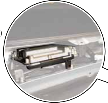
Motronic Engine Control Module (ECM) J220, under plenum chamber cover
