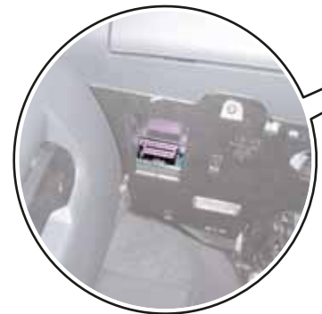
16-Pin Connector T16 on left side, beneath instrument cluster (DLC)
