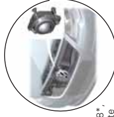
Distance Regulation Control Module J428*, behind the nameplate
