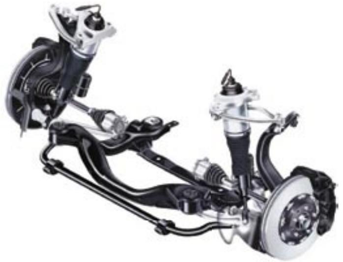
Harshness occurs when a vehicle vibrates from moving across road joints, projections, stepped differences, or depressions on paved roads. Driving on the expressway increases the pitch of the thumping sound. The impact force from the road surface causes the tires to vibrate. The tires transmit the vibration through the suspension system to the car body. Harshness has a frequency of 30 to 60 Hz.
