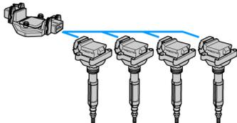
Power Output Stage N122 and Ignition Coils
