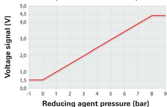
Voltage-pressure chart (transmission function)
