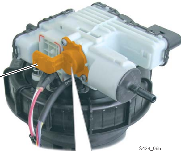
Reducing Agent Metering System Pressure Sensor G686
