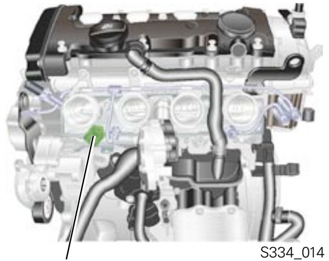
Fuel Pressure Sensor G247, High Pressure System
