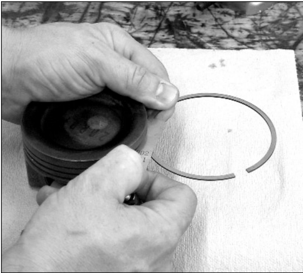
Flat-blade feeler gauge being used to measure piston ring clearance.
