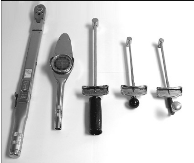
Types of torque wrenches include, from left, “click” type, dial type, and three versions of the basic beam-type.
