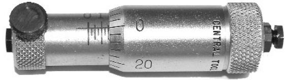
Typical inside micrometer, most often used to measure inside dimensions such as bore diameter. Note: the micrometer shown reads in non-metric units.
