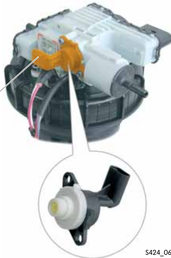
Pressure sender for reducing agent metering system G686
