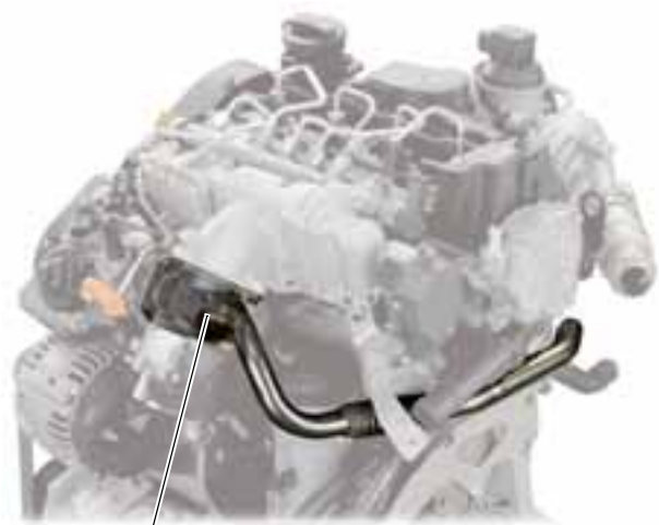
Exhaust gas recirculation valve N18
