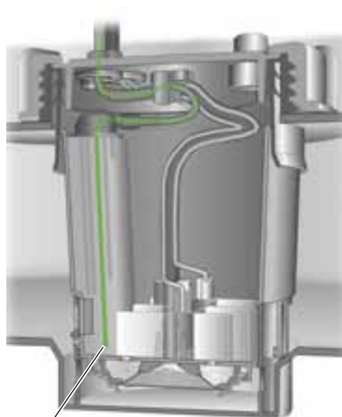
Temperature sender for reducing agent G685
