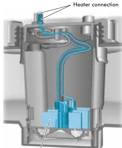
Heater for reducing agent tank Z102
