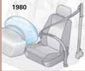
Front airbag - driver airbag, belt tensioner - front passenger side
