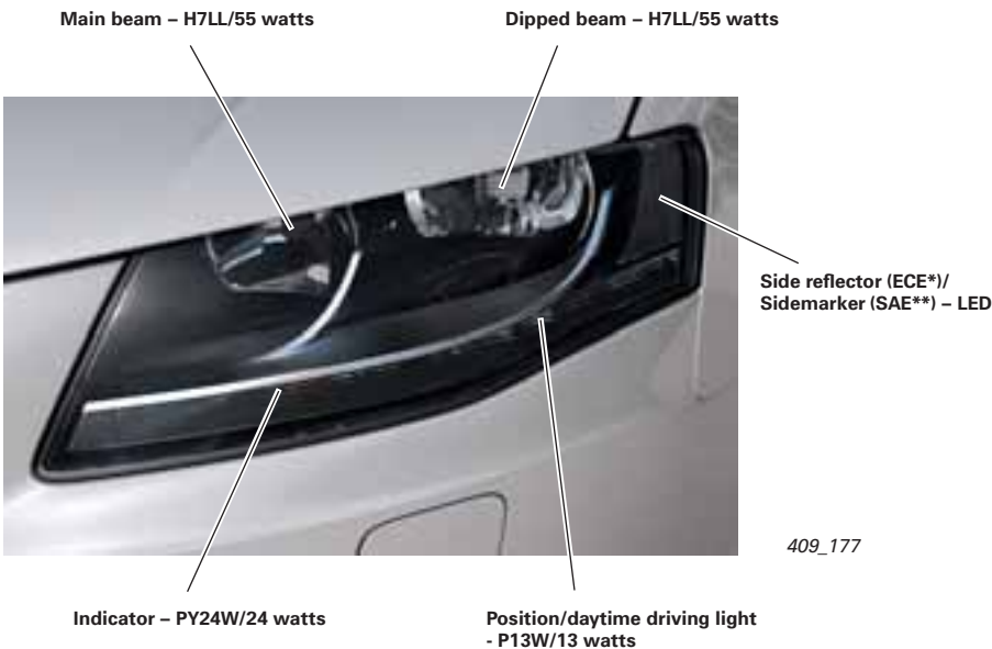
Lamp configuration in the halogen headlight version
