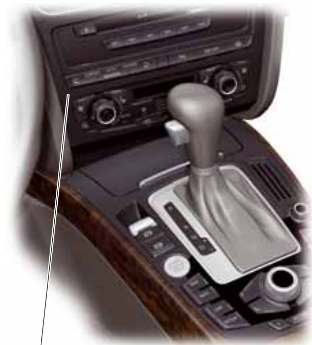
Operating unit -Audi drive select Charisma switch module E592
