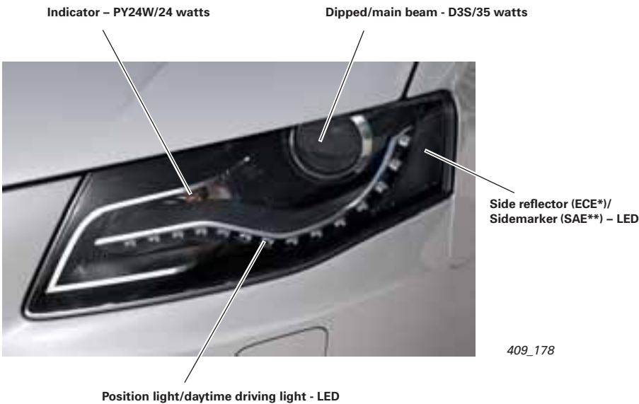
Lamp configuration in the bi-xenon version and in the bi-xenon version with adaptive light
