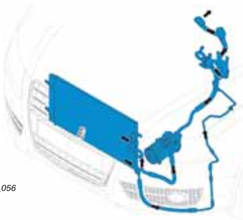
Coaxial line (low and high pressure lines combined in a single line)
