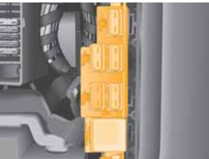
Additional fuse holder on left-hand side of luggage compartment
