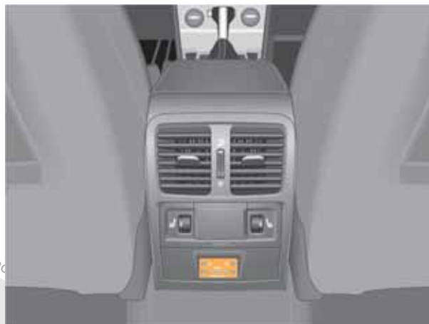
Location of additional connections unit R176
