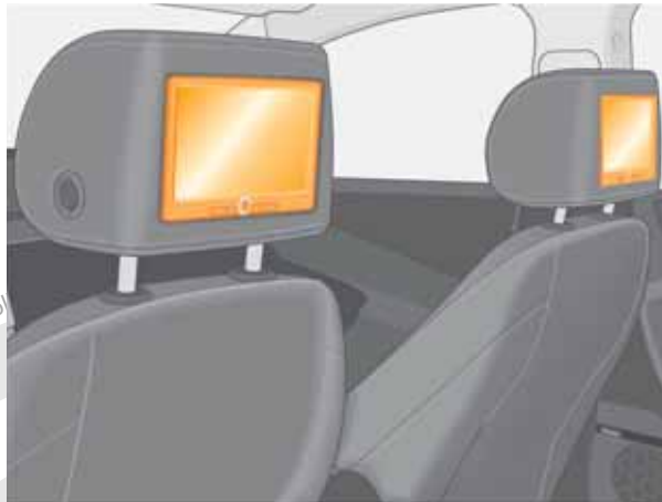
Locations of display units Y22 (left) and Y23 (right)
