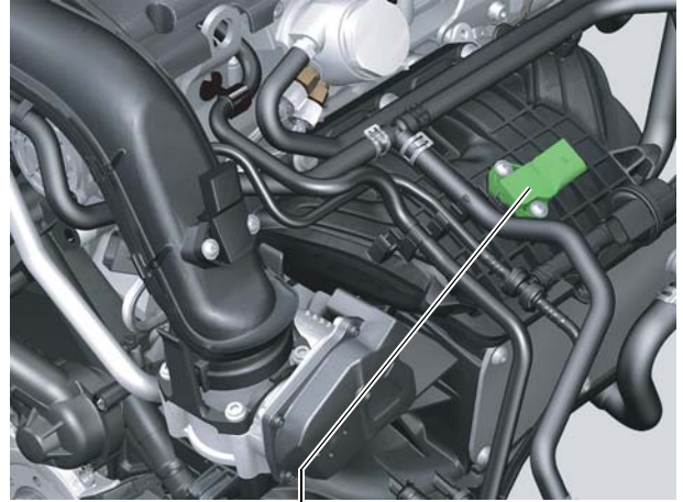
Intake manifold pressure sender G71 S405_044 with intake air temperature sender G42
