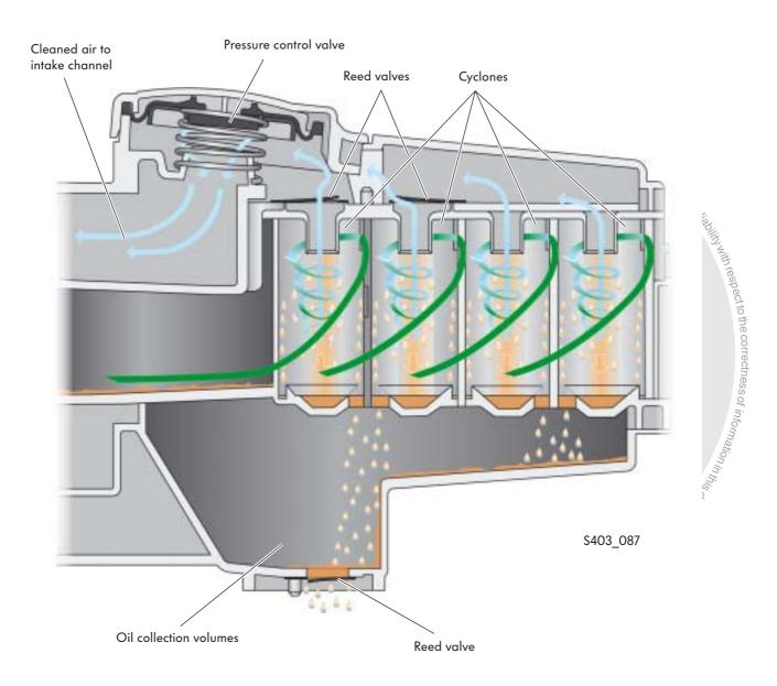
When the engine has stopped, a reed value opens that is closed by the higher pressure in the cylinder head while the engine runs. The oil passes from the collecting chamber to the oil sump via the cylinder head.
