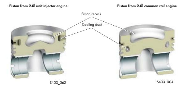
To cool the piston ring area, the pistons are equipped with an annular cooling duct, into which oil is sprayed via piston spray nozzles.
