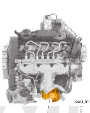
Throttle valve module J338 with throttle valve potentiometer G69
