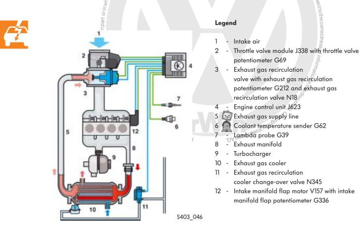
The exhaust gas recirculation quantity is controlled according to a map in the engine control unit. The engine speed, injection quantity, intake air mass, intake air temperature and the air pressure are taken into consideration.
