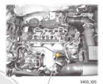
Exhaust gas recirculation cooler change-over valve N345
