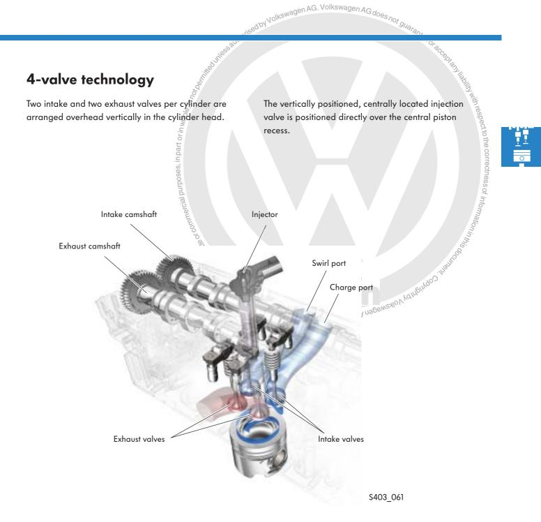
The shape, size and layout of the intake and exhaust ports ensure good volumetric efficiency and a favourable gas cycle in the combustion chamber.
