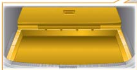
Large storage compartment in the luggage compartment floor - cover folded completely forwards
