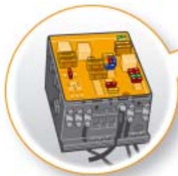
Pre-fuse box on the left in the engine compartment
