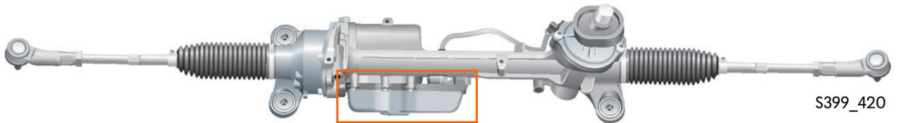
The control unit is cemented and screwed to the steering box. The control unit contacts are welded to the electric motor and can therefore not be separated. By using the steering box casing for thermal dissipation, there is no temperature-related reduction in the steering assistance even when a very high level of heat develops in the control unit.
