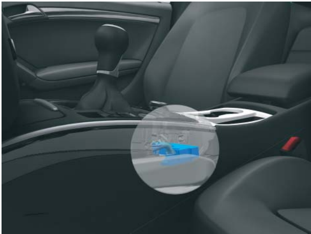
Installation location the R138 aerial in the centre console 393_015
