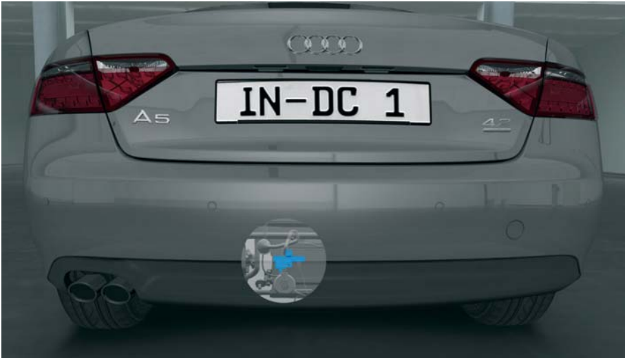
Installation location of the R137 aerial in the luggage compartment 393_016
