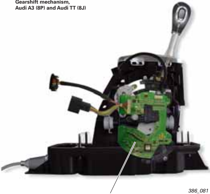
Selector lever sensor system E313
