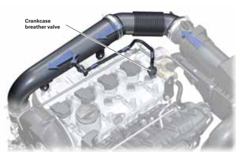
Cutaway view of crankcase breather valve
