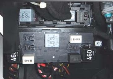
**Onboard power supply control unit**
