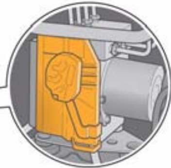
ABS control unit J104, on the left in the engine compartment
