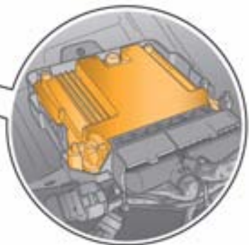
Engine control unit J623, on the left in the engine compartment
