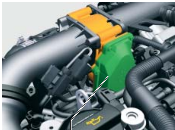
Regulating flap control unit J808 with regulating flap potentiometer G584
