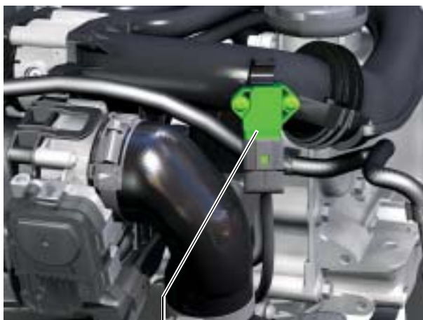
Intake manifold pressure sender G583 with intake air temperature sender G520
