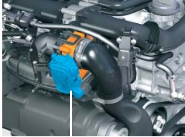
Throttle valve module J338 with throttle valve drive G186
