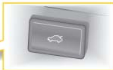
Button to close rear lid in luggage compartment E406
