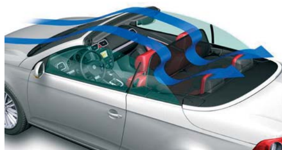
Airflow with wind deflector
