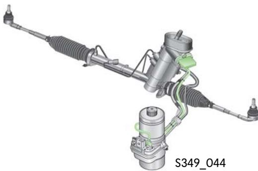
The hydraulic pump for the electro-hydraulic power steering is driven by an electric motor. The power steering is thus not dependent on the operating state of the vehicle engine and the energy supplied for steering assistance is adjusted to requirements. This ensures an improvement in comfort when manoeuvring and helps save fuel.
