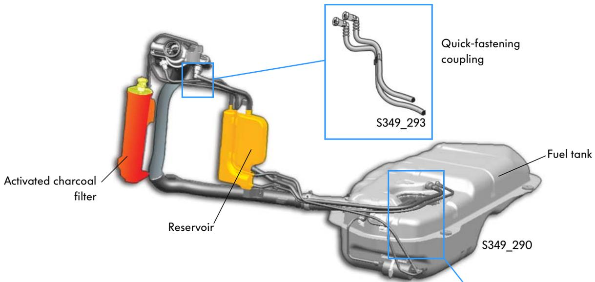
The activated charcoal filter is located in the rear right wheel housing.
