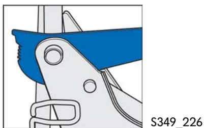
The backrest is locked by four teeth at the same time to distribute the force.
