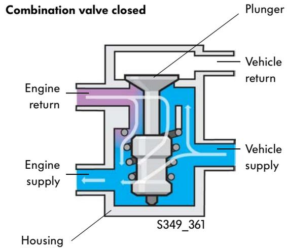
As the engine temperature increases, the fuel temperature in the engine return also increases. This heats the plunger with the wax element in the combination valve. The wax element then expands and pushes the piston upwards against the spring.
