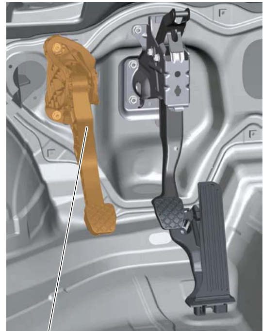
Clutch pedal with clutch position sender
