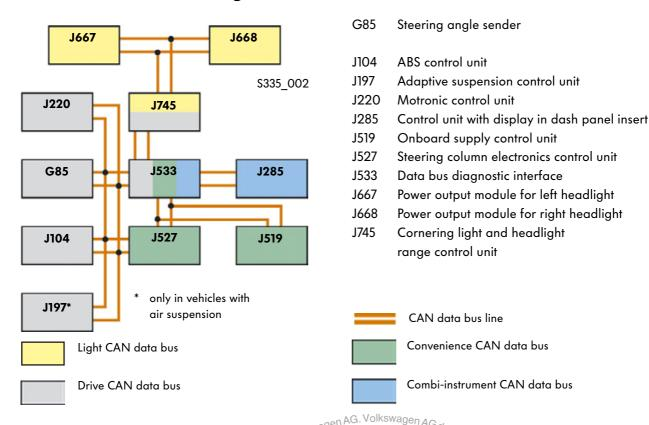
The picture shows the control units used for the cornering light functions and the CAN network. Data is exchanged between the control unit for headlight range control J431 and the power output modules in the left J667 and right J668 headlights via a 500 kBaud CAN (light CAN data bus). This light CAN data bus is a separate CAN data bus and is not connected to the 500 kBaud drive CAN data bus. The light CAN data bus also does not run via the diagnosis interface for data bus 533.
