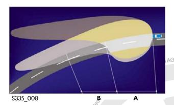
The diagram clearly shows the improved illumination of the road when the vehicle is cornering. The darker light cone represents the illumination with a conventional dipped beam.
