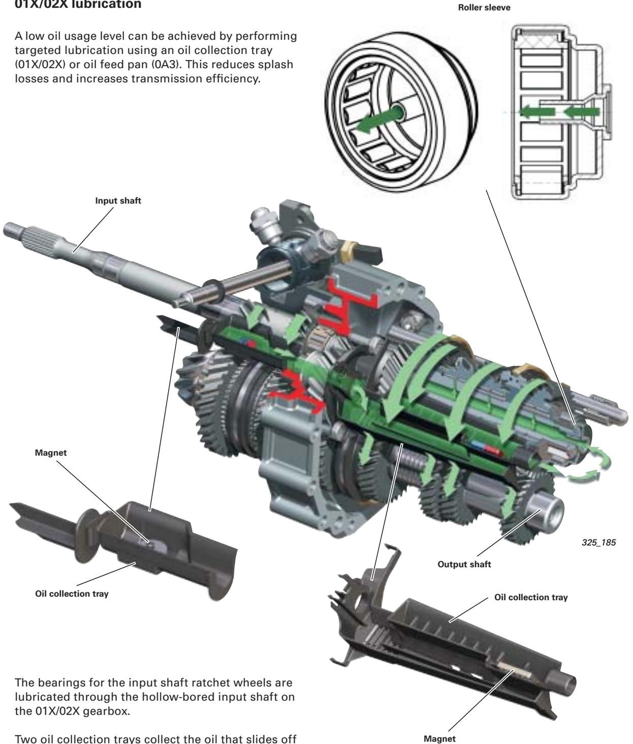
The bearings for the input shaft ratchet wheels are lubricated through the hollow-bored input shaft on the 01X/02X gearbox.
