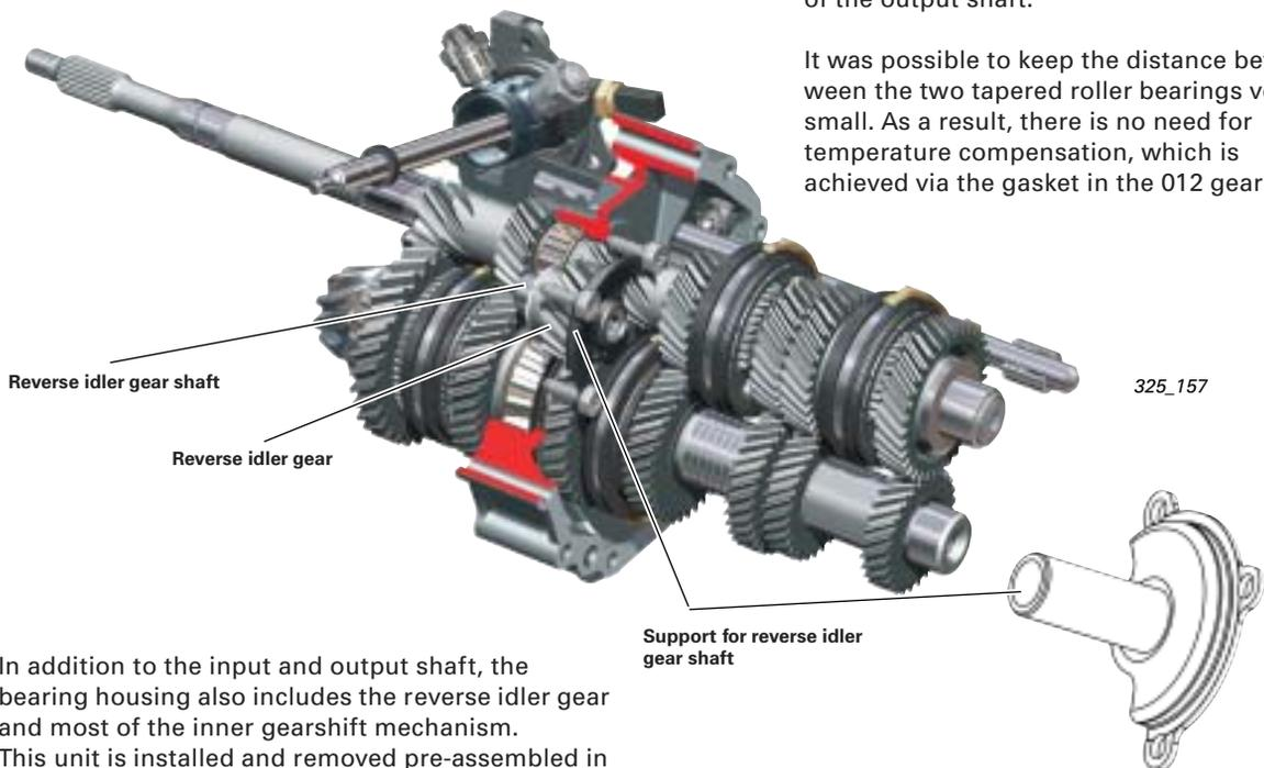
In addition to the input and output shaft, the bearing housing also includes the reverse idler gear and most of the inner gearshift mechanism. This unit is installed and removed pre-assembled in this way.
