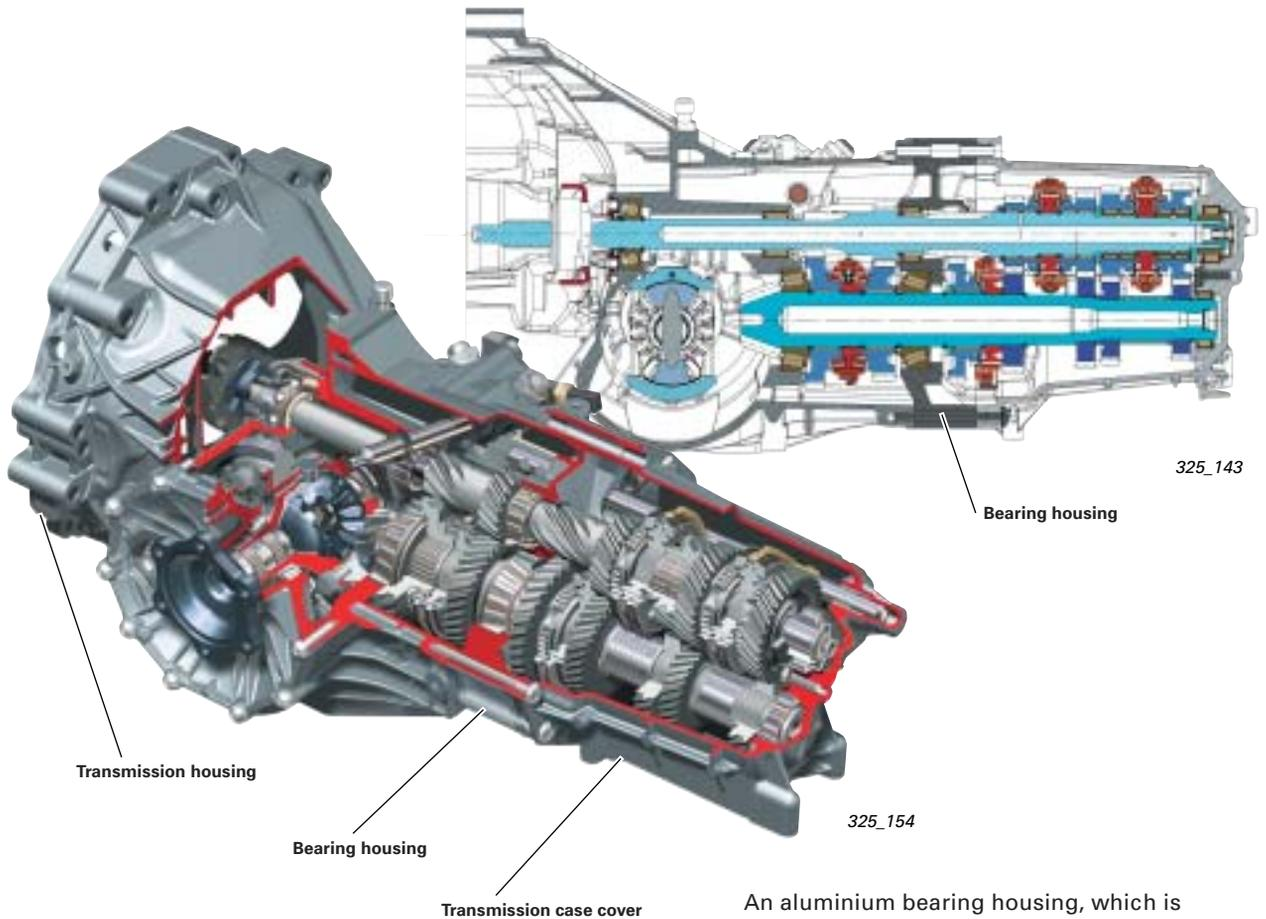
An aluminium bearing housing, which is screwed in between the transmission housing and the transmission case cover, was developed for the 01X and 02X gearboxes.
