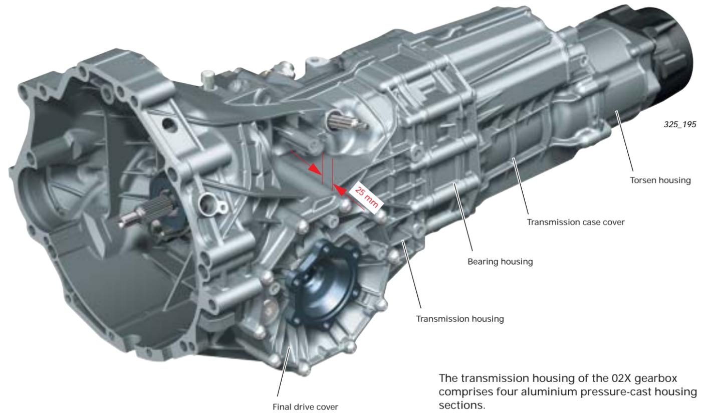
The transmission housing of the 02X gearbox comprises four aluminium pressure-cast housing sections.
