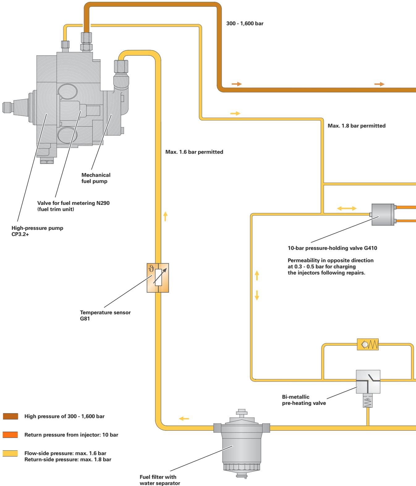
The injection pressure has been increased to 1,600 bar, which is 250 bar more than in earlier 2nd generation common-rail systems.
