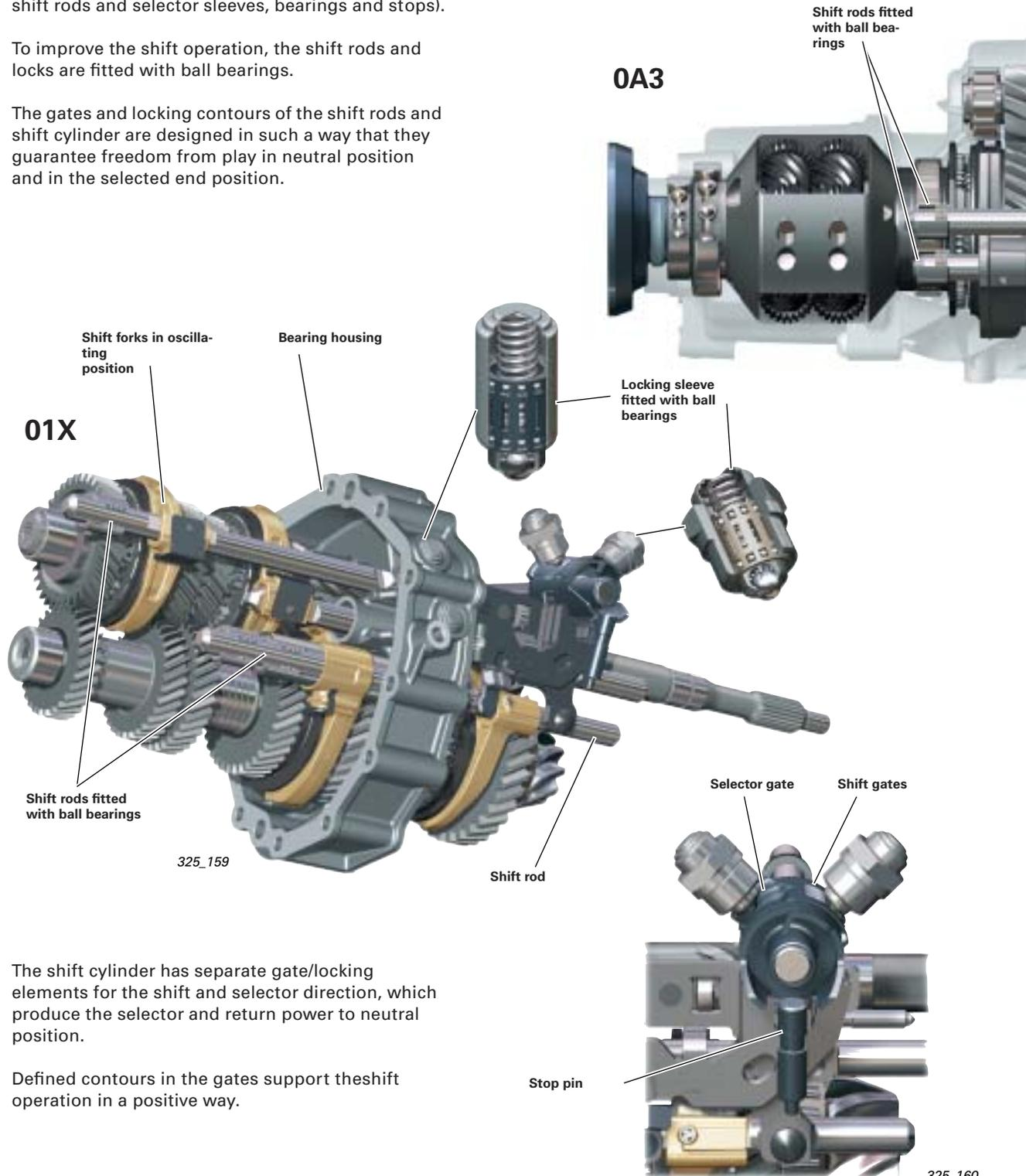
The shift cylinder has separate gate/locking elements for the shift and selector direction, which produce the selector and return power to neutral position.
