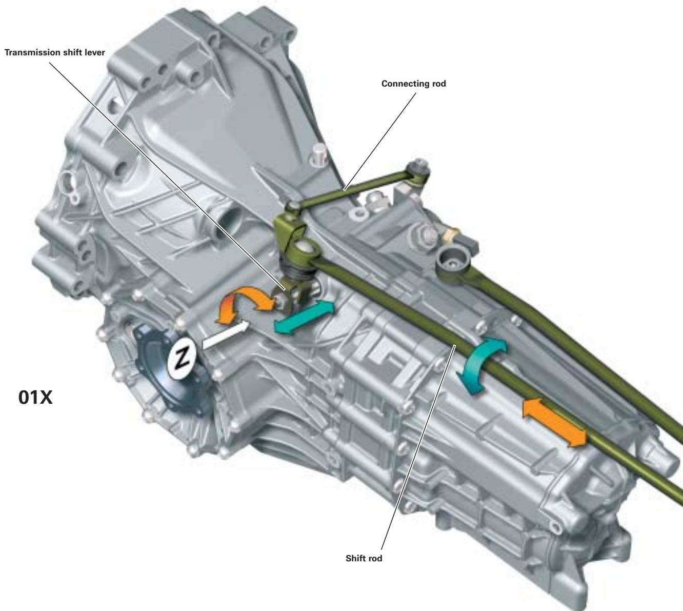
The fundamental design of the gear selector (outer gearshift) for the 01X/02X and 0A3 gearboxes is the same.
