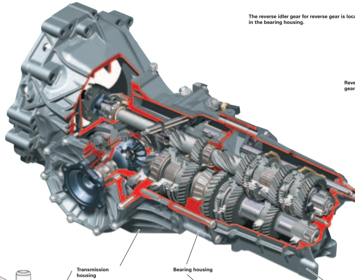
The reverse idler gear for reverse gear is located in the bearing housing.
