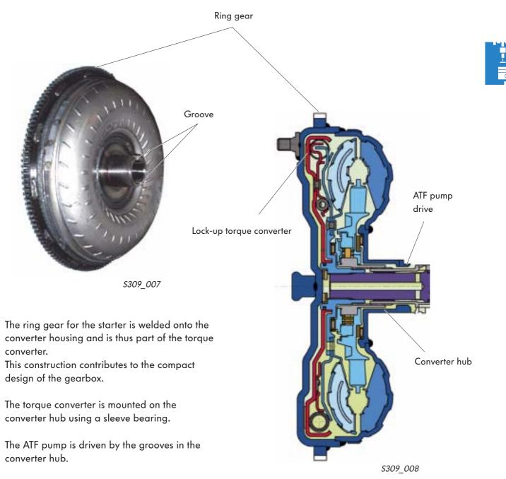
Different converter types are used to adapted the gearboxes to the characteristics of the different engines.
