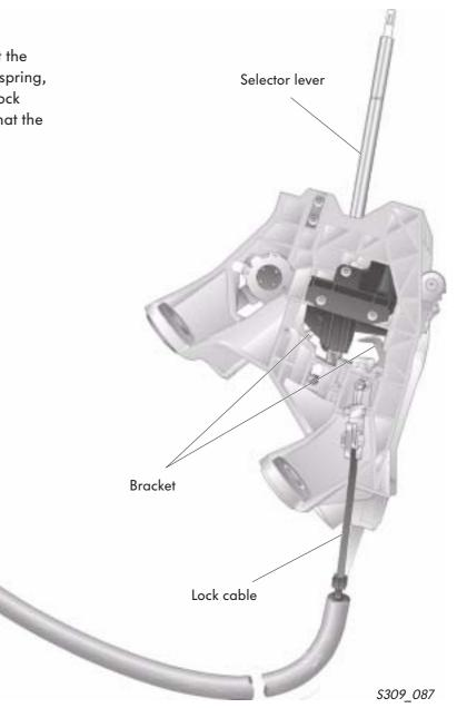
Moulded section on lock cable The release button on the selector lever lifts the pull rod when you move the lever. This allows the selector lever to be moved in the gate. When you release the button, the pull rod is locked into the new position again by the spring.
