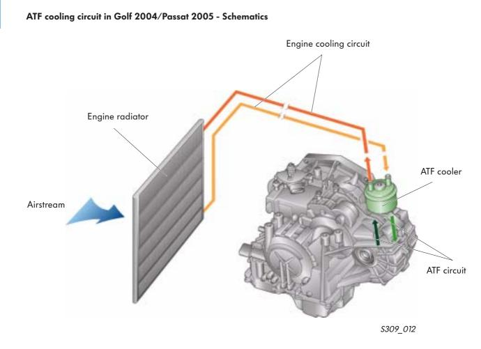
The "closed ATF system" does not need to be topped up nor does the ATF level have to be checked. There is no need to disconnect the ATF lines when the gearbox is removed or fitted.
