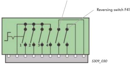
Switches 1 to 4 for selector lever positions
