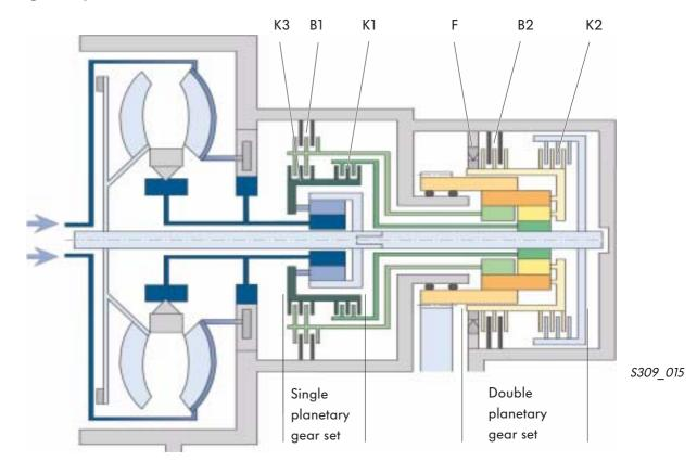
The planetary gear set uses a Lepelletier construction.
