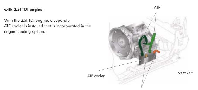
Engine cooling circuit
