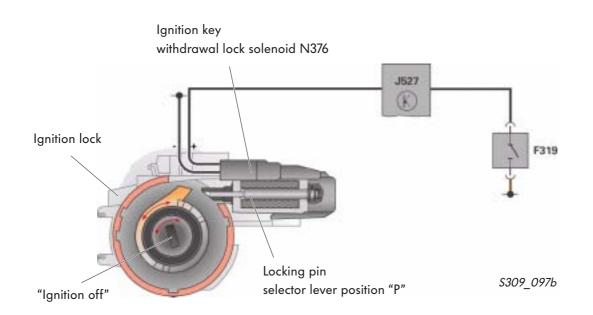
Selector lever in drive position, the ignition is switched on
