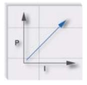
Pressure control valve with rising characteristic curve N90 and N91
