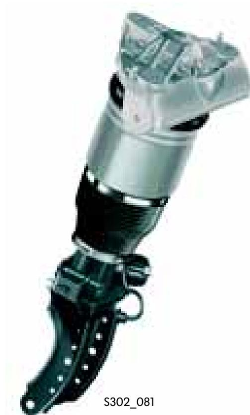
The air suspension is combined with a controllable vibration damping system.
