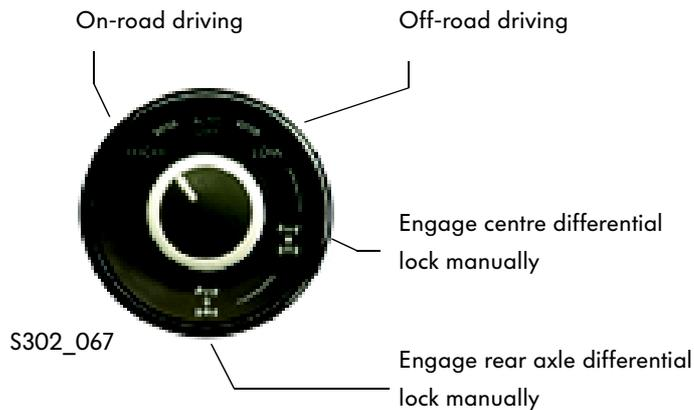
The **"HIGH"** setting is for on-road driving. The differential locks are engaged automatically depending on the situation (e.g. icy conditions). In this case, the differential lock is not closed to 100%, as for example with a constant mesh coupling, but is engaged with a soft setting. The off-road reduction stage is not engaged.
