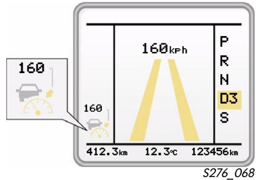
If a *relevant* vehicle is detected, it appears in the display. The colour of the kph display changes to grey since the displayed speed no longer matches the actual speed.
