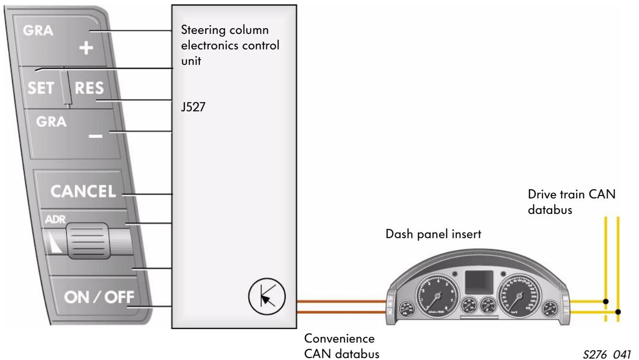
The APC system is mainly operated by means of the left button cluster on the multi-function steering wheel. However, the brake and accelerator pedals, as well as the gear selector lever position, also have an influence on the APC system.
