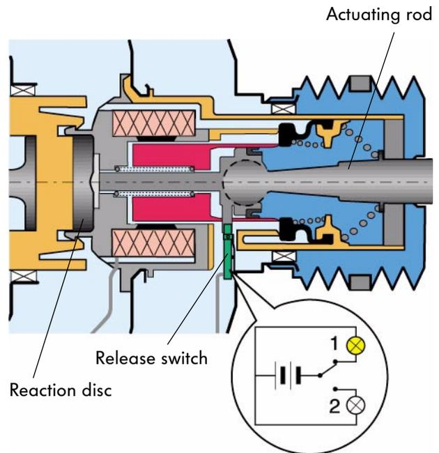
If the driver applies the brake, pressure is applied to the reaction disc via the actuating rod. The reaction disc is compressed. The release switch rises from the brake servo housing. Electric circuit 2 is closed.
