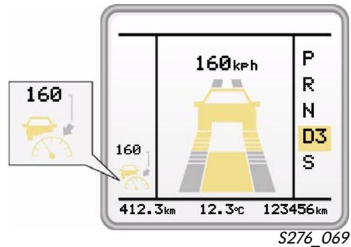
The *time gap* (following distance) to the vehicle in front is represented in seven steps. The time gap actively set by the driver is represented in orange. The centre bar indicates the vehicle's position in relation to the vehicle ahead.
