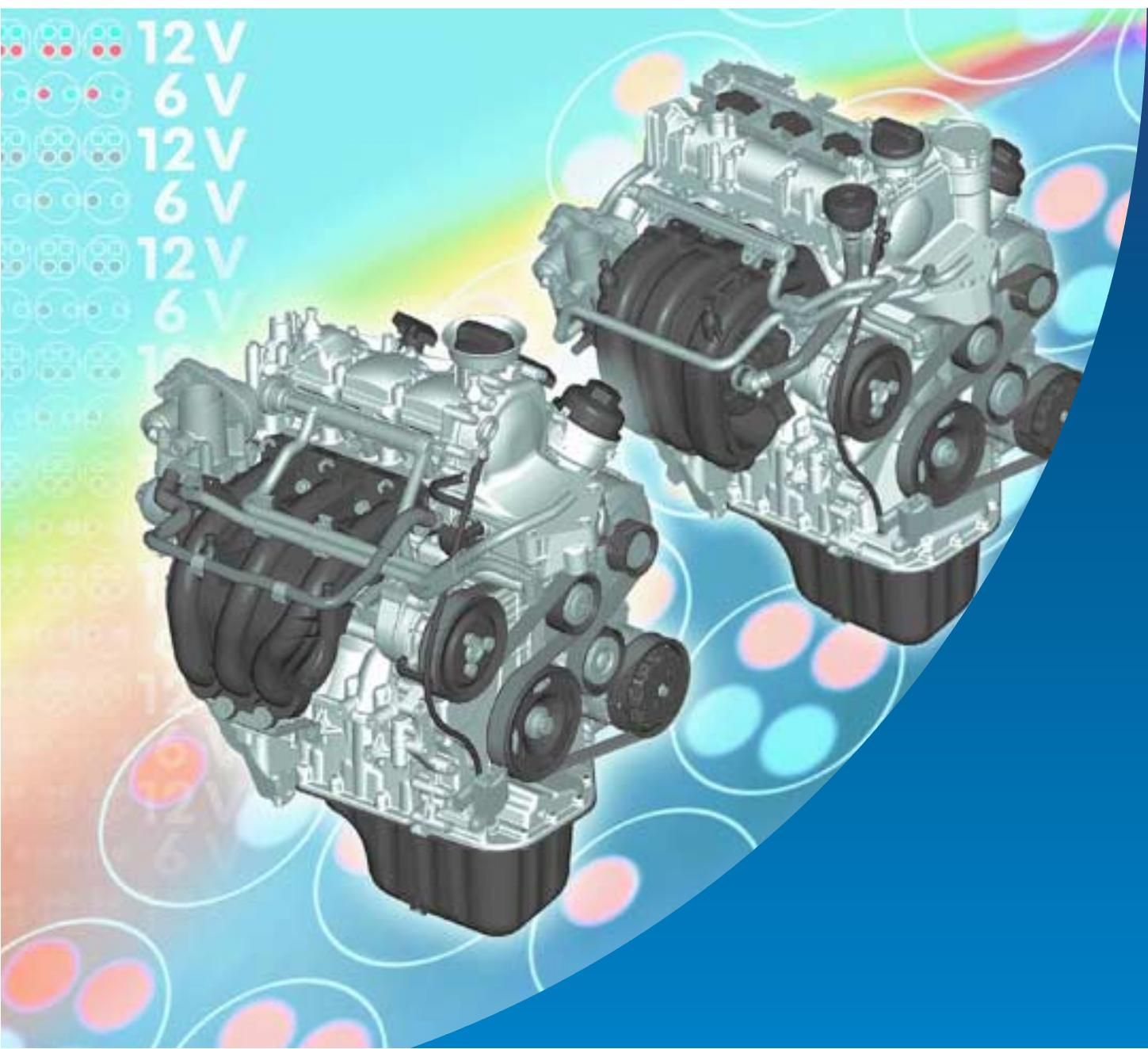
The two 1.2 ltr. engines mark the introduction of 3-cylinder petrol engines at Volkswagen. This pair of entry-level engines rounds off the range of engines of the 2002 Polo.
