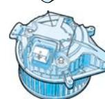
Series resistor for fresh air blower N24, control unit for fresh air blower J126 with fresh air blower V2
