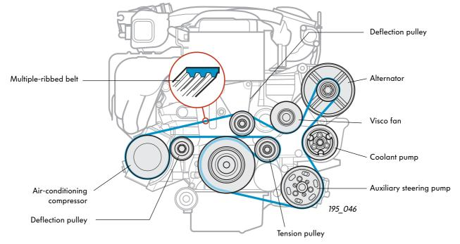
In the longitudinally mounted engine the coolant pump is located on the auxiliary holder. As a result, this engine is slightly shorter than the transversely mounted engine.
