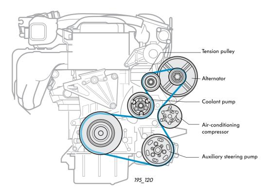
In the transversely mounted engine the coolant pump is integrated in the cylinder crankcase.
