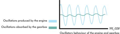
Oscillatory behaviour of the engine and gearbox at idling speed
