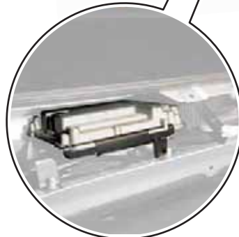
Motronic Engine Control Module (ECM) J220, under plenum chamber cover
