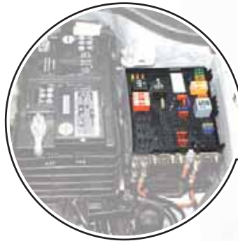
Fuse and relay center under hood on driver side SB
