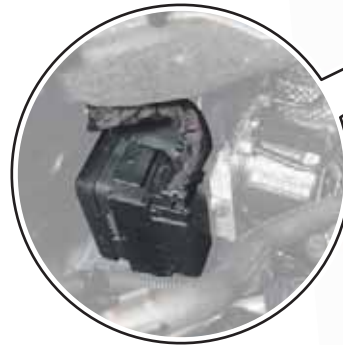
ABS Control Module J104, on right side of bulkhead, in engine compartment
