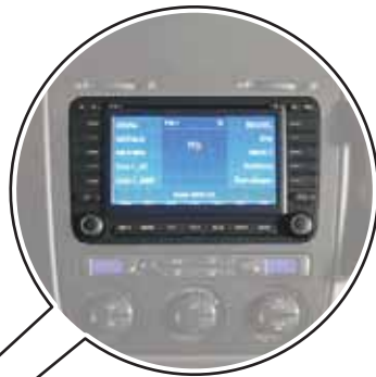
Radio/Navigation Display Control Module J503 or Radio R, in center console
