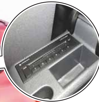
CD Changer R41, in center console, beneath front armrest
