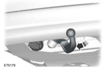
Move the tow ball arm to the operating position. The tow ball arm automatically locks in the operating position. The locking process is clearly audible and the warning tone will stop.
