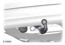
The tow ball arm automatically swivels into the lowered position.
