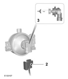
**Note:** You cannot separate the fog lamp bulb from the bulb holder.
