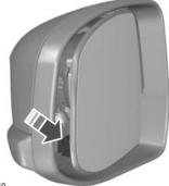
1. Insert your fingers into the gap between the mirror housing and the mirror glass and pull gently to remove the mirror glass.
