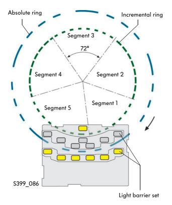
The incremental ring is divided into 5 segments each with 72° and is read by a light barrier set. The ring is broken inside the segment. The sequence of the openings is the same within a segment, but different between the segments. This results in the coding of the segments.
