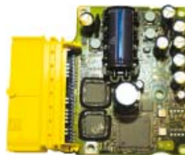
Airbag control unit J234 – housing open
