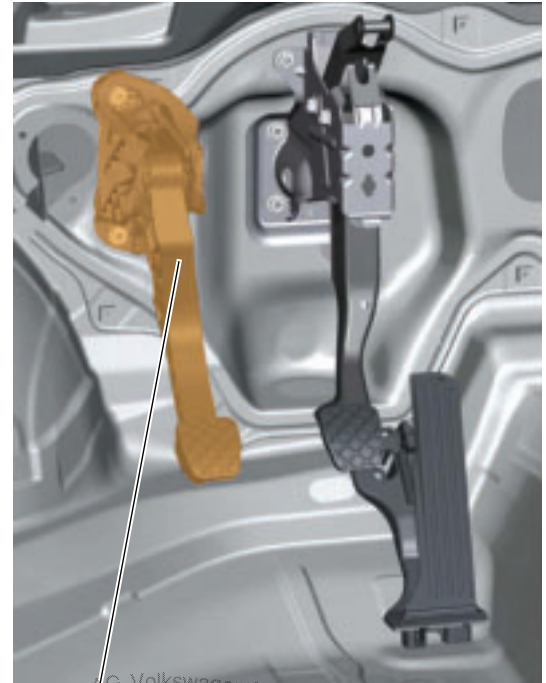
Clutch pedal with clutch position sender
